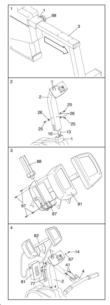
5. Connect the Reed Switch Wire (13) and the two Extension Wires (41) to the corresponding wires on the Console (8).
